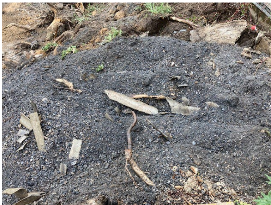
Plate 1: Example ash fill material with ACM
