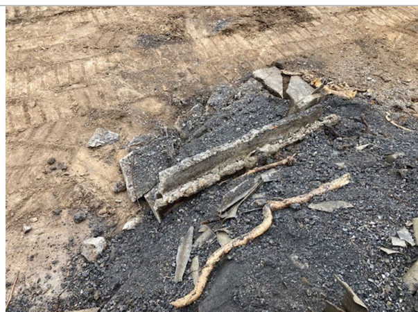
Plate 5: Examples of ACM in fill material
